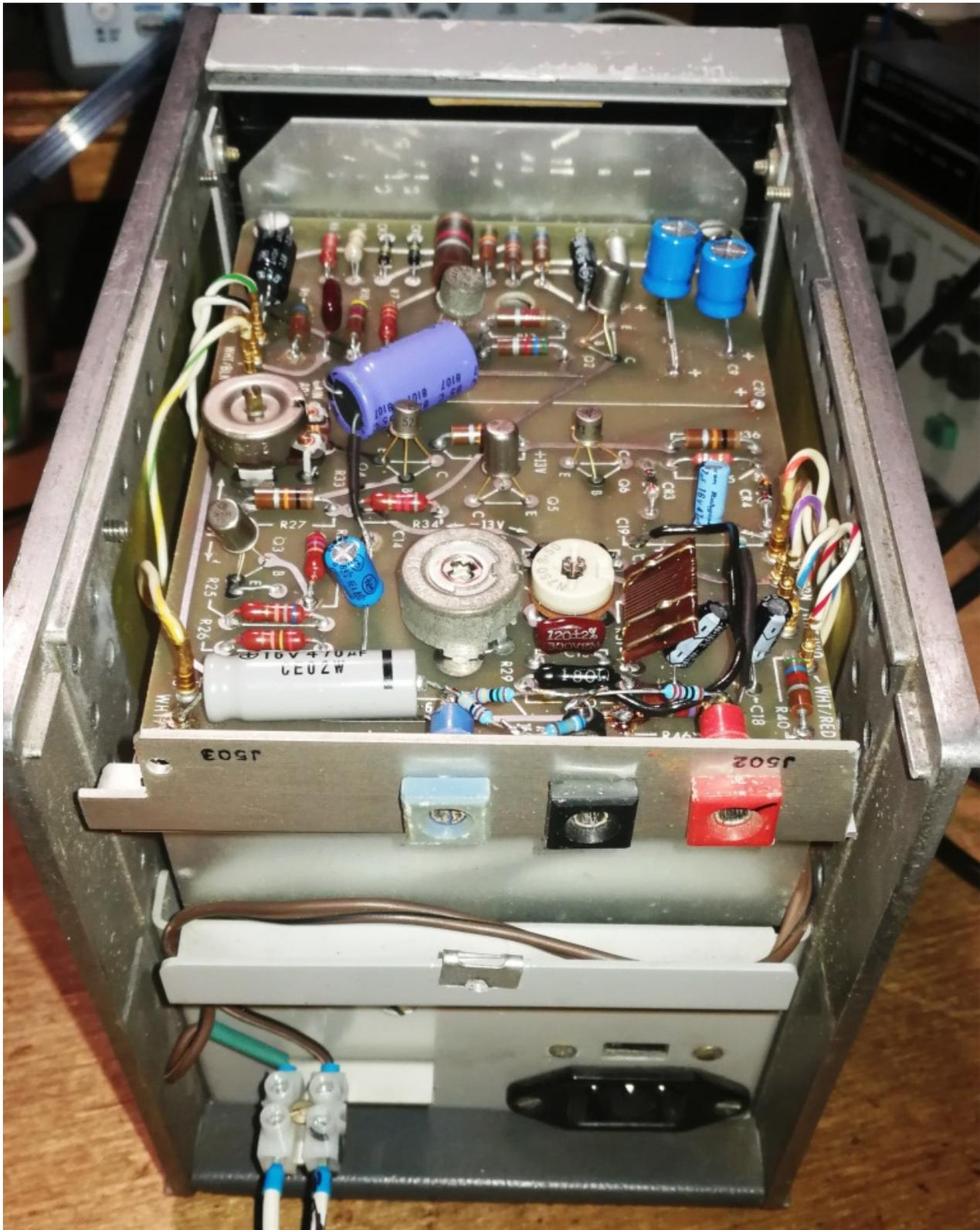
Rear view showing external DMM connections, and external battery connection
