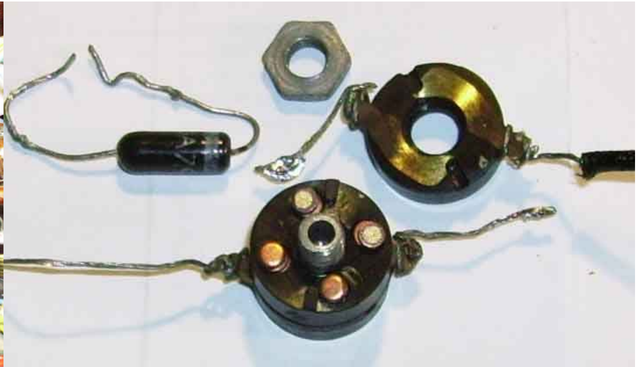
Copper oxide diode bridge in Paton Electrical VCT2 Valve Tester
