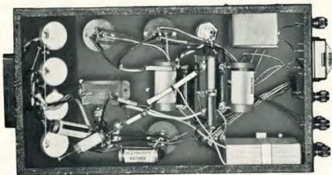
Fig. 2. Under-chassis view of the amplifier shown in Fig. 1. To ensure stability all leads have been kept as short as possible and well spaced. Note the screened grid lead running from the input circuit to V1.
