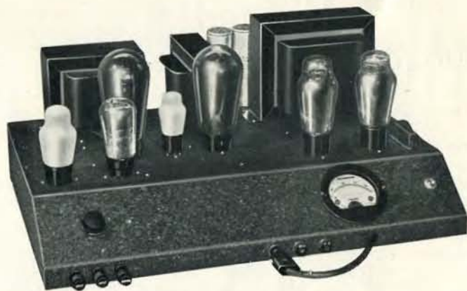
Fig. 5. The Partridge 45w. Amplifier Design, as interpreted by Messrs. H. J. Leak & Co. The equipment is easily transportable and is also suitable for large permanent installations or radio relay work. The large output of 45 watts is obtained without the use of an excessively high H.T. voltage.
