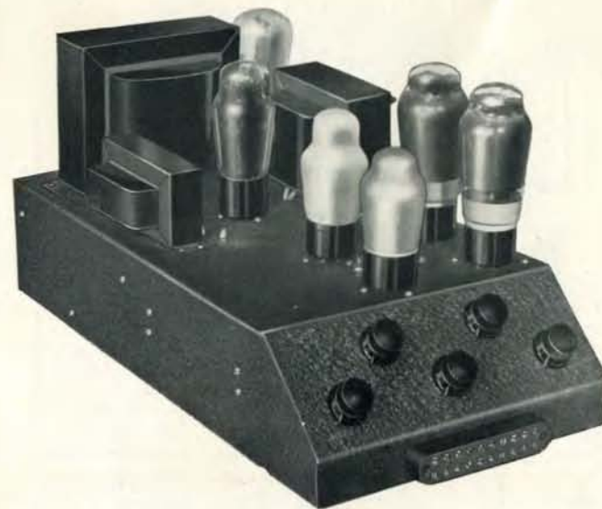
Fig. 3. The Partridge Economy 28, as built experimentally for the author by Messrs. H. J. Leak & Co. This was the first amplifier to employ the Partridge Control Circuit (invented by N. Partridge, B.Sc., A.M.I.E.E., patent rights purchased and controlled by The Mullard Radio Valve Co., Ltd.). An undistorted output of 28 watts is obtained although the cost, size and weight are no more than those of the usual 12 watt chassis.
