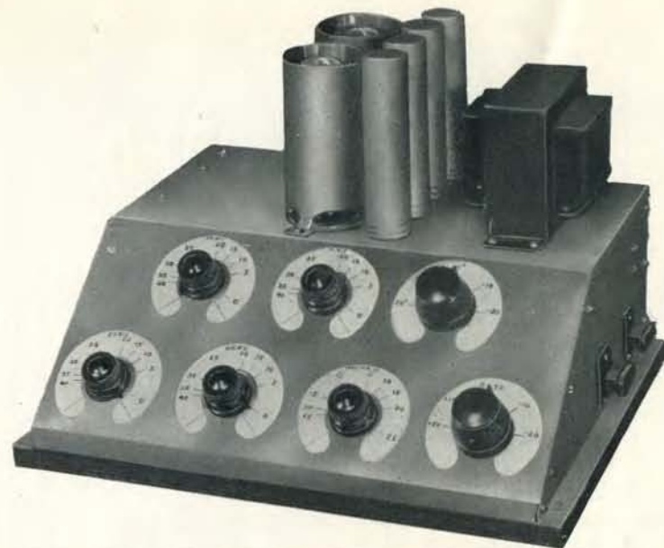
Fig. 8. The Partridge Two-Stage Pre-Amplifier. This is the ideal control unit for use in conjunction with the Partridge 30w. or 45w. amplifiers. Two microphones and two pick-ups together with separate bass and treble tone controls can all be operated from the sloping panel.
