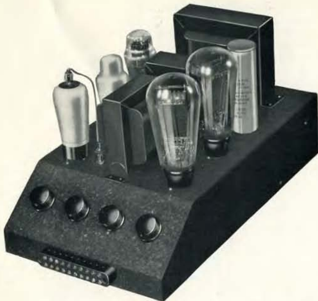
Fig. 1. The Partridge 12w. P.A. Amplifier as built by Messrs. H. J. Leak & Co. The mains transformer is at the back of the chassis and the intervalve transformer as far from it as possible at the front of the chassis, the cores of these components being at right angles. The chassis is of steel, but stout aluminium is equally effective and reduces the risk of unwanted magnetic coupling.
