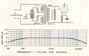
Fig. 12. The circuit diagram and response curve of the Partridge Microphone Transformers Types M250/350 and M400/600. Note that the primary is split into two equal sections so that the line may be balanced with respect to earth.
