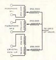
Fig. 16. A satisfactory circuit for mixing a sensitive pick-up with insensitive microphones (see text).
