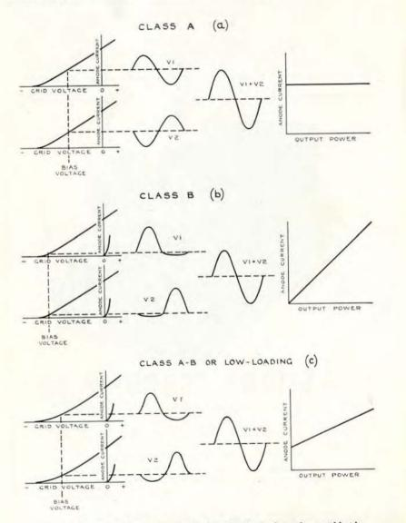
Fig. 4. Illustrating the operation of push-pull output valves when working in Class A, Class B and Class A—B (low loading). The transformer design and grid-bias are the factors governing the manner in which the valves function.
