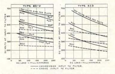
Fig. 9 Characteristic curves of the American 83V and 5Z3 rectifiers when operated in the circuits of Fig. 10 (a) (full lines) and Fig. 10 (b) (dotted lines).
