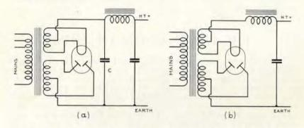
Fig. 10. (a) illustrates the usual condenser input to the smoothing filter, while (b) shows the choke input circuit that has to be used where good H.T. regulation is essential.
