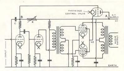
Fig. 5. The Partridge Control Circuit. Invented and provisionally patented by N. Partridge, B.Sc., A.M.I.E.E., patent rights purchased and controlled by The Mullard Radio Valve Co., Ltd.
