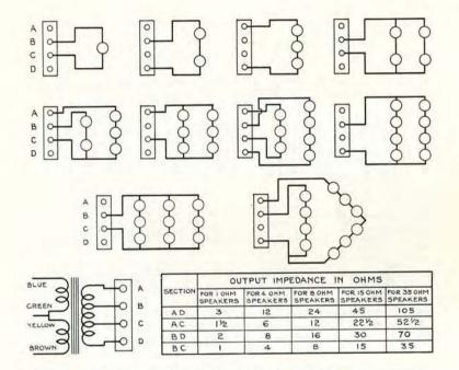
Fig. 19. Method of employing the Series Type Partridge Output Transformer. This scheme can be applied to any output valves, and speakers of any impedance, but all the speakers must be of the same impedance.
