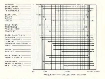
Fig. 2. Audible frequency range of various sources of sound. The crosses mark the cut-off points that are just detectable by the average person.
