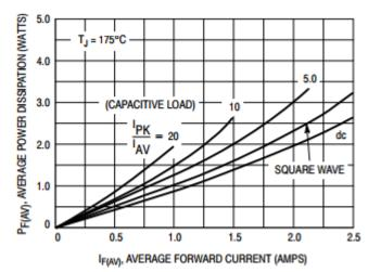
**Figure 2.** MUR160 power dissipation versus forward current, from [4].
