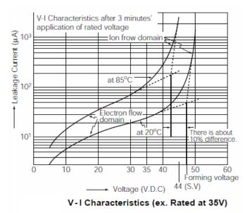
Figure 31. Leakage current characteristic versus voltage [17].
