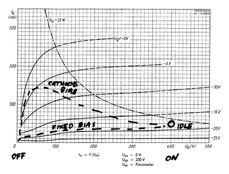
Figure 25. Example turn-on loci for hot output stage valves.
