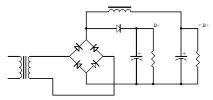
**Figure 30**. Capacitor and choke input filtered rails from same diode bridge.
