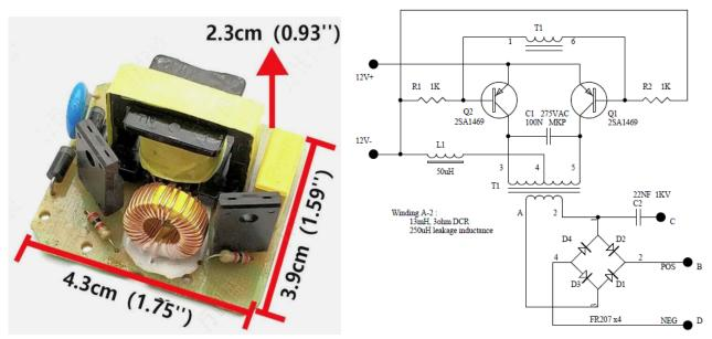
Figure 40. '35W' Baxandall inverter module with included bridge rectifier.
