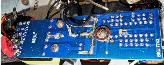
Figure 39. '150W' inverter module with added rectifier/filter.
