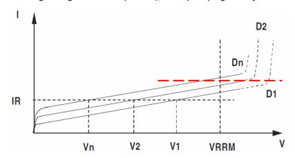
**Figure 12.** Graphical representation from [6] of diode leakage current dispersion.
