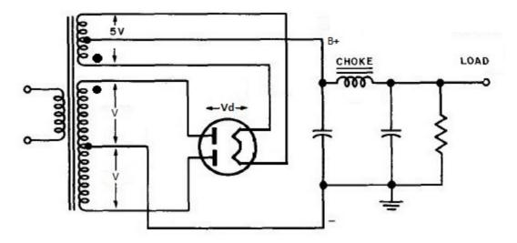
Figure 33. Typical power supply circuit with 5V centre-tapped heater winding.
