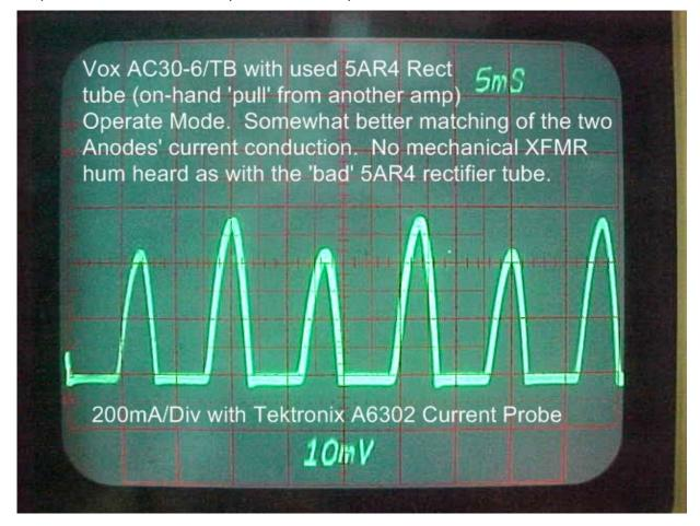
Figure 35. Rectifier current pulses on CT connection.
