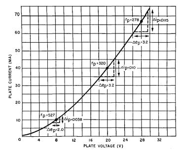
Figure 14. 6H6 valve diode V-I curve from [8].
