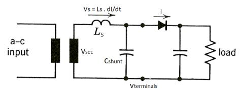
**Figure 16.** Equivalent circuit showing secondary winding with transformer voltage Vsec, leakage inductance (Ls) and shunt capacitance (Cshunt).
