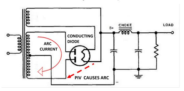
**Figure 38.** Illustration of arcing current in diode causing low resistance across transformer secondary winding.
