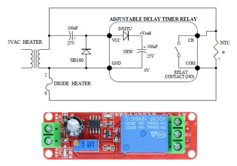
Figure 27. Common eBay adjustable delay timer relay switch module.
