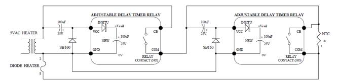
Figure 28. Adjustable delay timer relay switch modules for heater in step sequence.
