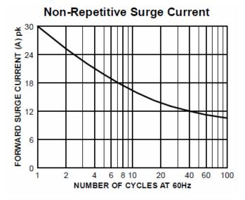
**Figure 9.** IN4007 surge current capability, from datasheet.
