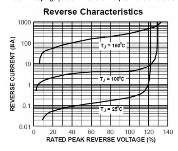
**Figure 8.** 1N4007 reverse current versus inverse voltage, from datasheet.
