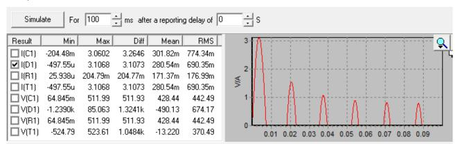
Figure 23. PSUD2 results showing hot turn-on I<sub>apt</sub> level of 3.1A for GZ34.
