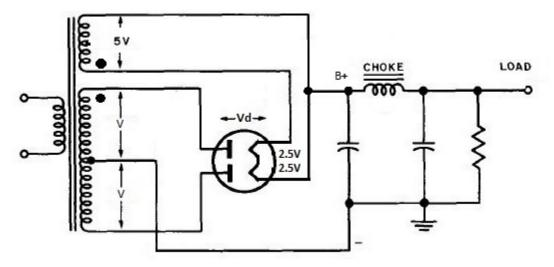
Figure 34. Typical power supply circuit with 5V heater winding (no centre tap available).
