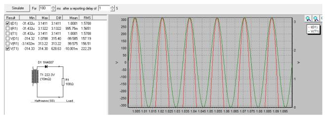
Figure 1. IN4007 simulated current waveform (red) for datasheet continuous current rating.
