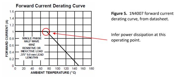
So the 1N4007 power dissipation Pd in Figure 5 can be inferred by noting the expected thermal resistance Rth (from MUR160), and calculating Pd =  $(150^{\circ}\text{C} - 75^{\circ}\text{C})/\text{Rth}$ . For 0.375" lead lengths, the MUR120 indicates Rth  $\sim 84^{\circ}\text{C/W}$  (although this could be increased somewhat given a higher Tamb and a lower Tj for the 1N4007 operating conditions). Hence from Figure 5, 1N4007 Pd  $\sim 0.9\text{W}$  for 1A lav, Tamb=75°C and Tj=150°C.
