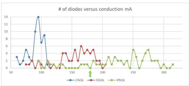
Figure 37. Number of diodes in batch with mA anode current levels (5mA span).
