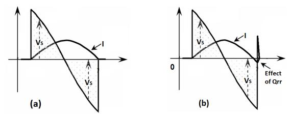
**Figure 17.** Voltage across secondary winding leakage inductance Ls due to changing winding current I with ideal diode (a), and when diode Qrr is significant (b).
