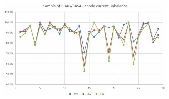
Figure 36. Anode current imbalance for a batch of 5U4G/5AS4 rectifier diodes
