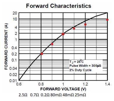
Figure 24. 1N4007 diode characteristic with PSUD2 model values.
