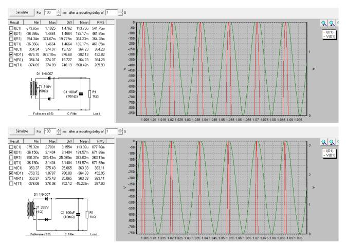
Figure 4. IN4007 simulated current waveform (red) for capacitor input circuit examples.
