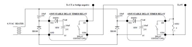
**Figure 29**. Adjustable delay timer relay switch modules for CT link in step sequence.
