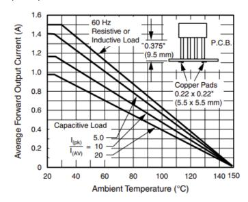
**Figure 7.** Vishay W10G forward current derating curve, from datasheet.
