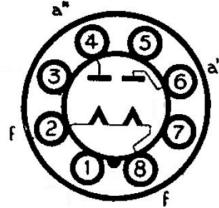
Figure 32. Directly heated filament configuration.
