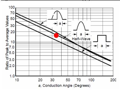
**Figure 13.** Graphical representation from [1] of diode conduction angle for different peak to average current ratios. For single phase rectifiers the maximum conduction angle is 180 degrees.
