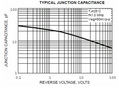
Figure 18. UF4007 diode junction capacitance for reverse voltage.
