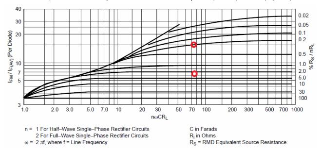
**Figure 3.** Schade's curve for peak current to average current ratio from [1], with 2 power supply operating points identified.
