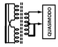
**Figure 20.** Snubber arrangement for full-wave rectified power supply as commonly found in tube amps, along with Mark Johnson's recommended 'Quasimodo' test-jig setup [9].
