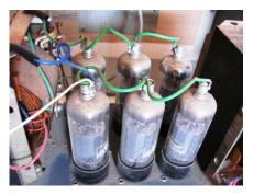
Be careful with 6CM5 /EL36 valves in Philips PA amps, as they were often crammed together, had no bias adjustment, and variation in idle conditions between valves cannot be checked. Although they can cope with high anode dissipation, stressing each valve with >12W anode idle power and cranked screen current is risky with used valves, unless circuit changes are implemented.
