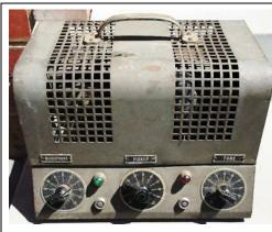
Circa 1952; unbranded; uncommon mic sockets on front; no mains fuse or switch.
