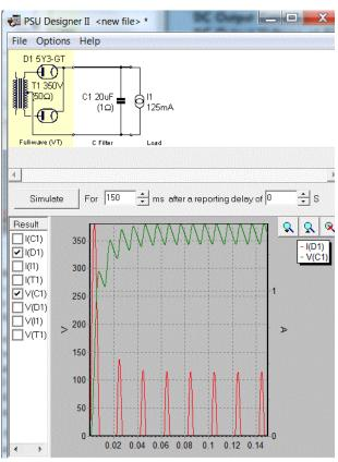
When modifying part values, PSUD2 will give an alert if a peak current limit is exceeded. Preferably cross check that the current limits are the same as in the datasheet.
