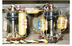
Some valve base spigots have a 'tree' attachment to simplify the local connection of parts without having to use connecting wire to nearby tag boards. The photo shows an example of tree spigots.
