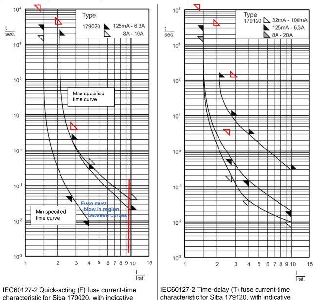
Figure 1. Indicative fuse current – time curves at min/max specifications.
