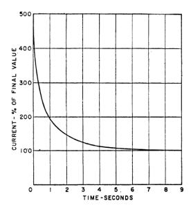
Figure 7. Heater current response.
