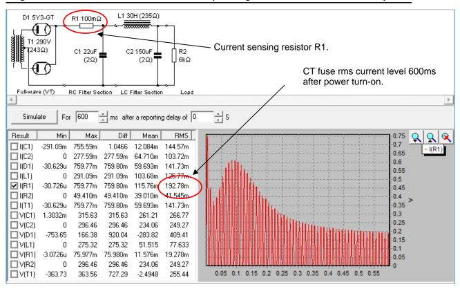
Figure 5. PSUD2 simulation screen example for CT fuse in 5W 6V6 SE amp.
