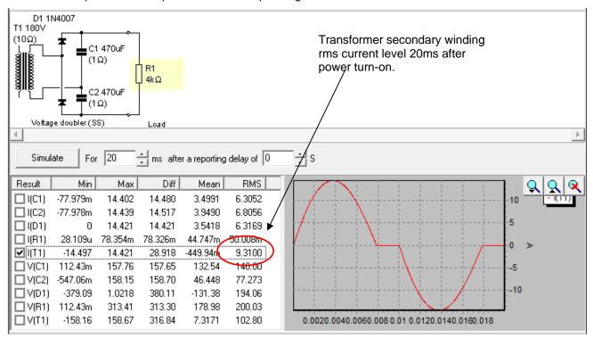
Figure 4. PSUD2 simulation screen example for VASE 100W KT88 PP fixed bias amp.
