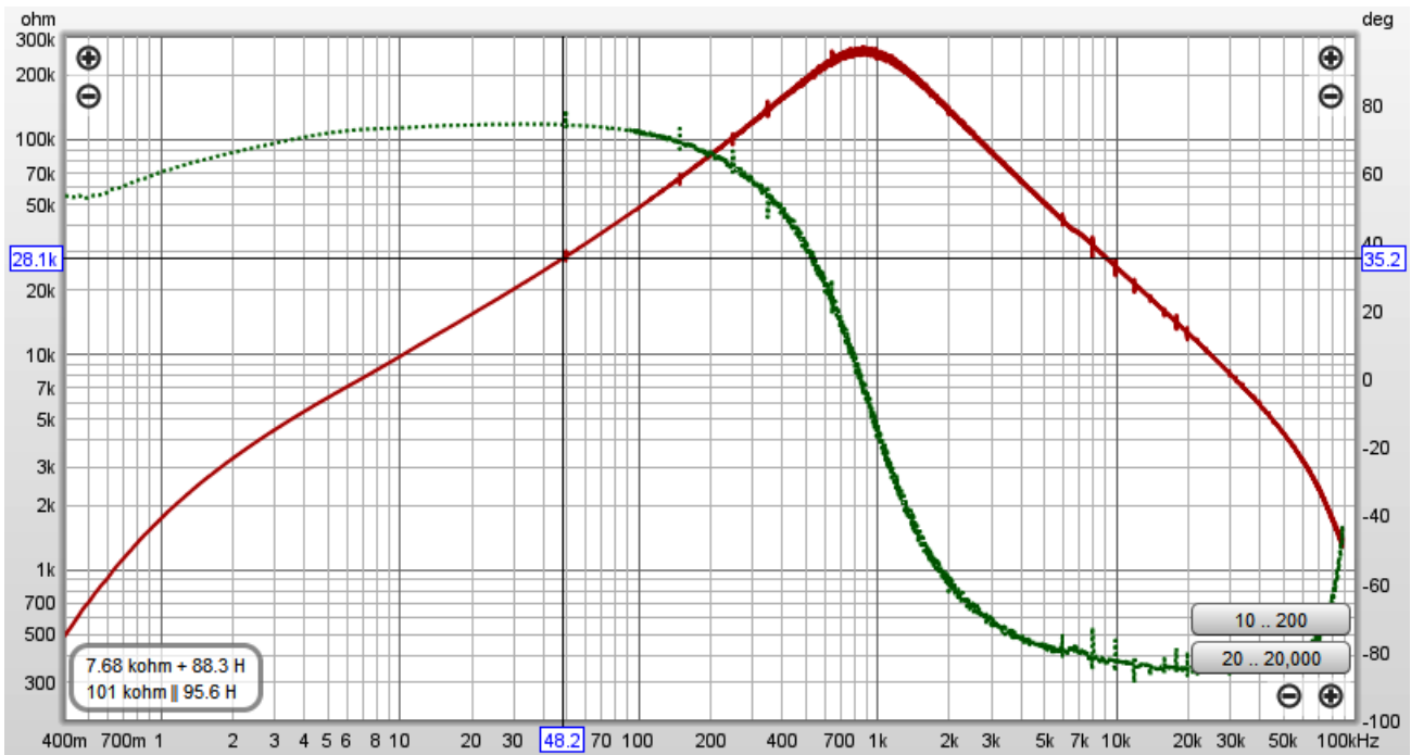
Figure 6. Primary winding impedance versus frequency at about 1.5Vrms for WWFB
