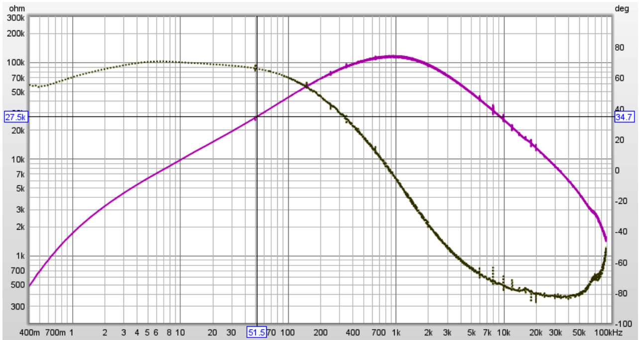
Figure 8. Primary winding impedance of WWFB with 8.5Ω secondary configuration.
