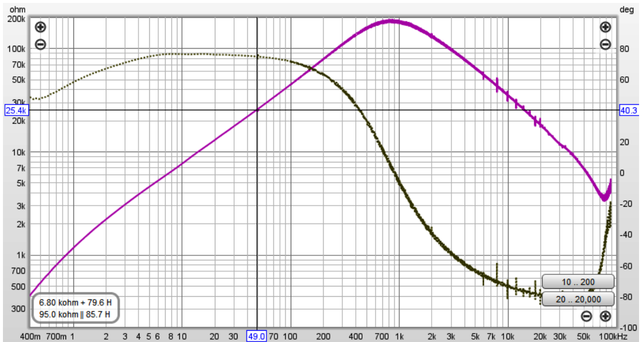
Figure 9. Primary winding impedance of Ferguson OP25 (new) with 4Ω secondary configuration.
