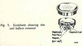
these were removed carefully from the magnet assembly, care being taken to prevent damage to the coil connections. Figs 1 and 2 show the coil before and after removal from the earphone.
